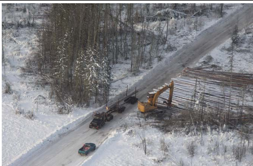
Photo #2: Tree length logs being loaded out using a hydraulic log loader with a butt n top attachment.
